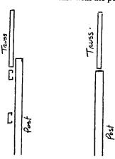
Post Between End Wall: Truss will set directly on top of post.
