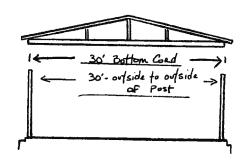
**Post Placement:** Considering the width of your building the outside width of the post will be the same distance as the bottom width of your truss. **Example:** 30' Truss
