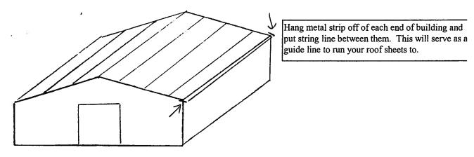
This will allow you to run your roof sheets down to the string each time you place sheet. You can watch how roof sheet goes to string and tell if sheets are going on squarely. As you install roof sheets you will run a roll of tacky tape (mastic) between each roof sheet joint. After the tacky tape has seasoned it will be attached to each sheet like welding the joints.
