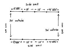
Example of Post Placement for Walls on 40' Long Building: This is basic post placement for side wall post. Span between side wall post will always be no more than 12' 6" so that trusses are not set more than 12' 6" apart. 10' centers are commonly how we figure our floor plans.
