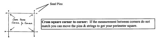
**Pins:** From this you will establish the actual corners of the building. You will need to cross square the string line to make sure your base is square. At this time you will drive steel pins in ground to mark where each post will be placed. Also placement of your doors should be marked.
