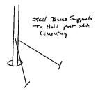
Tack weld support brace to post to hold level while cement settles. Pour concrete dry as possible so it will be firm around post.
